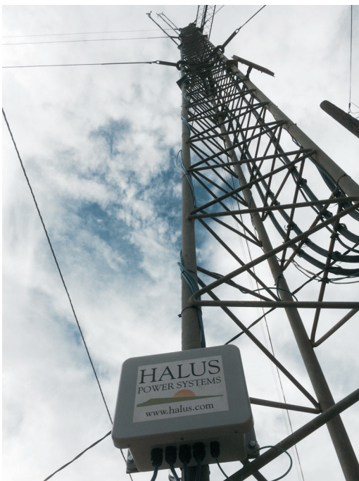
Hero Data Logger installation at strawberry farm in Central California.
